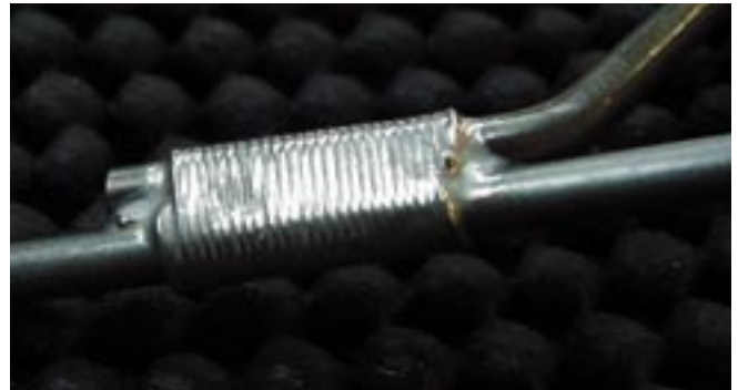
Silver solder is applied and heated until capillary action pulls the solder in to fill all the voids between and under the wire wrapping.
