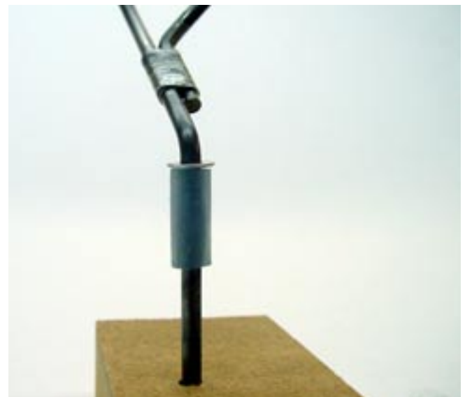
Here an inner wheel bearing surface is being added. A #4 washer has been placed on the axle and is supported by a short length of silicone fuel tubing. The fuel tubing is impervious to the acid flux and the soldering heat and will prevent solder from flowing through to the other side of the washer. A simple wood block is used as a supporting jig.
