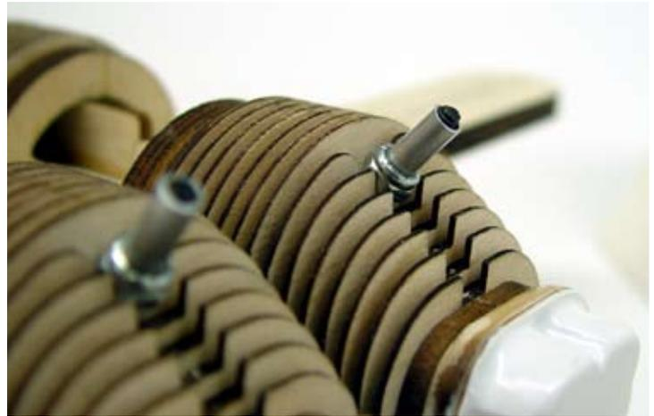
Below right, Rocker box covers and plugs installed with heat shrink plug wires. Left, the push rod tubes have been installed. Manifold tubes will be permanently installed after the cylinders are attached to the cowl.
